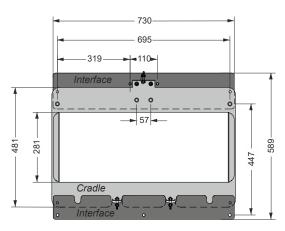
The integration of the PROPECHE Class V onboard is facilitated by the cradle (on which the container is fixed & secured) and its interface (fixed on deck). The container with cradle are easily removable for servicing as required by D227 French regulation.
